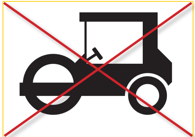
Picture 13: Installation equipment which cannot be used for compaction of manholes and chambers
