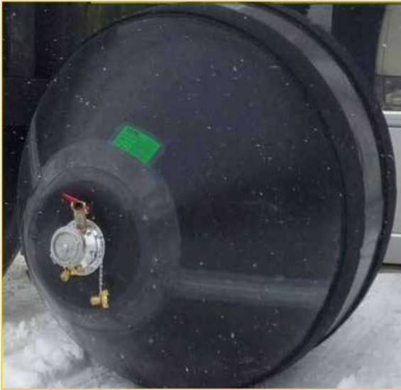
Shut-off bladders for manhole testing with additional air connection
