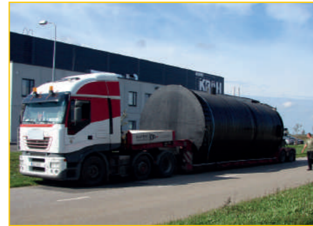
Transportation of a drinking water tank DN/ID 2000mm (79")
