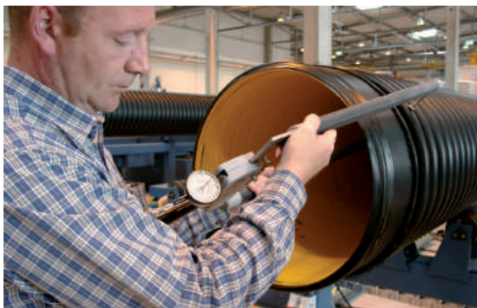
Checking of the wall thickness
