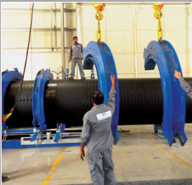
Butt-welding of pipes DN/ID 1800mm (71")
